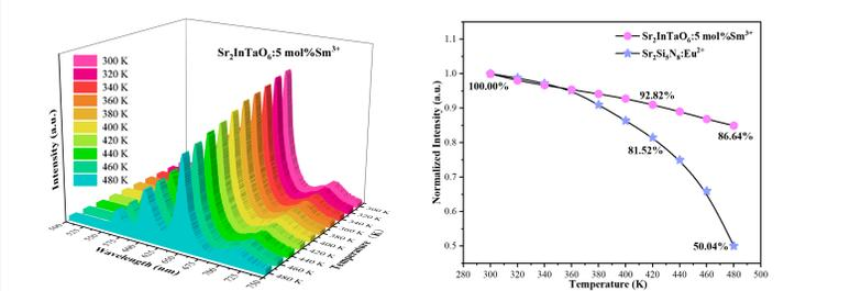
Fig. 7. (a) PL spectrum of  $\text{Sr}_2\text{InTaO}_6:5 \text{ mol}\% \text{Sm}^{3+}$  at 300–480 K. (b) Integral diagram of luminous intensity of  $\text{Sr}_2\text{InTaO}_6:5 \text{ mol}\% \text{Sm}^{3+}$  compared with that of commercially available red phosphor  $\text{Sr}_2\text{Si}_2\text{N}_8:\text{Eu}^{2+}$ .
