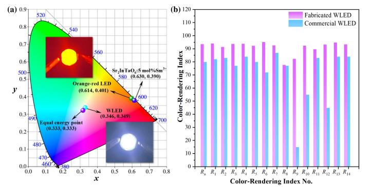
Fig. 10. (a) Coordinate diagram of  $\text{Sr}_2\text{InTaO}_6:5 \text{ mol}\% \text{Sm}^{3+}$  phosphor and the prepared LEDs. (b) Histogram of the CRI of the fabricated WLED compared with that of the commercial WLED.
