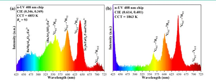
Fig. 9. (a) Electroluminescence (EL) spectrum of the WLED with a three-color method-based NUV chip. (b) EL spectrum of an orange-red LED based on a NUV chip.
