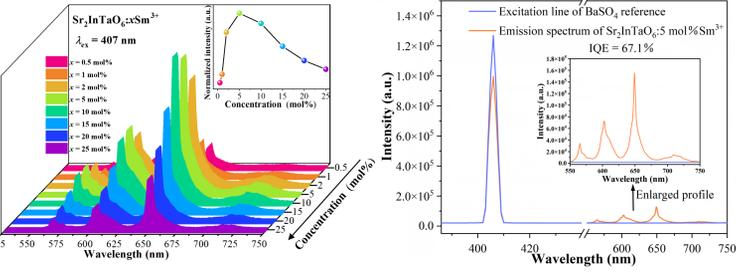
Fig. 5. Variation of  $\text{Sr}_2\text{InTaO}_6:\text{Sm}^{3+}$  fluorescence intensity with concentrations. Fig. 6. Excitation line of  $\text{BaSO}_4$  based and emission spectrum of  $\text{Sr}_2\text{InTaO}_6:5 \text{ mol}\% \text{Sm}^{3+}$  collected with an integrating sphere. (Inset: magnification of emission spectrum from 550 to 750 nm).
