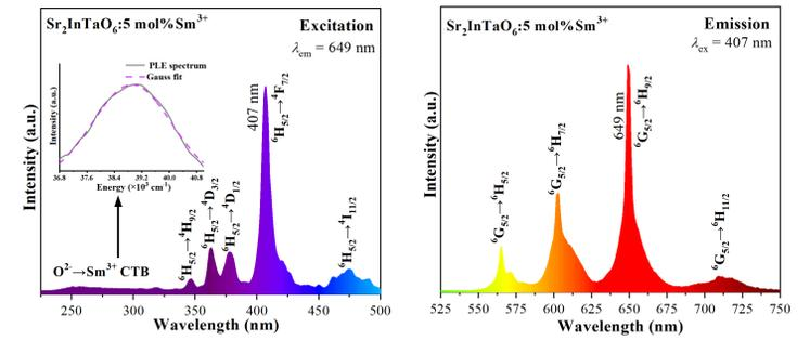
Fig. 3. Excitation spectrum of  $\text{Sr}_2\text{InTaO}_6:5 \text{ mol}\% \text{Sm}^{3+}$  ( $\lambda_{\text{em}} = 649 \text{ nm}$ , inset: Gauss fit result of CTB). Fig. 4. Emission spectrum of  $\text{Sr}_2\text{InTaO}_6:5 \text{ mol}\% \text{Sm}^{3+}$  ( $\lambda_{\text{ex}} = 407 \text{ nm}$ ).
