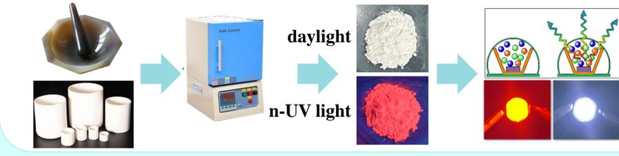
The synthetic raw materials for  $\text{Sr}_2\text{InTaO}_6:\text{Sm}^{3+}$  phosphor were weighed  $\text{SrCO}_3$ ,  $\text{In}_2\text{O}_3$ ,  $\text{Ta}_2\text{O}_5$ , and  $\text{Sm}_2\text{O}_3$  mixed in a mortar, and ground thoroughly. The mixed compounds were first sintered at 600 °C for 6 h, followed by secondary grinding and sintering at 1300 °C for 6 h, waiting for the temperature to drop to room temperature to obtain the target phosphors.
